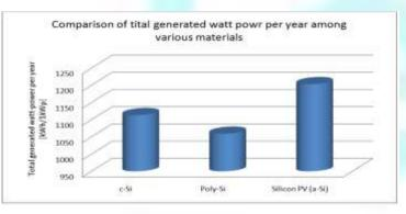
Assuming that the total solar radiation per year (1.323kWh/m2) is 100%, Silicon PV Modules can produce 90.95% of actually generated watt-power, about 80 to 84% higher than that of other crystalline silicon PV Modules.
