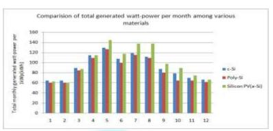
Crystalline-Si PV modules lose some power-generating capability with rises in temperatures. But Amorphous-Si PV modules can deliver maximum performance during summer when the electricity is needed most for air-conditions in houses and offices.
